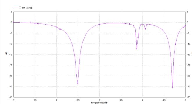
Fig 3.S-parameter versus frequency (return loss)
