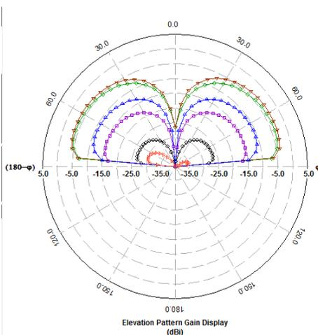
Fig 5.Radiation pattern at frequencies 2.5 GHz, 3.8 GHz, 4.7 GHz
