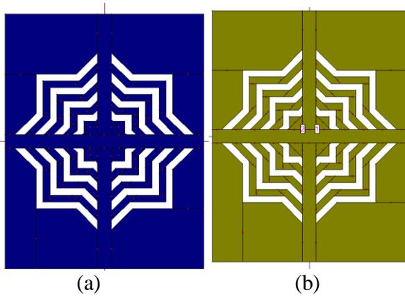
Fig1. (a) patch (b) patch with dual feed
