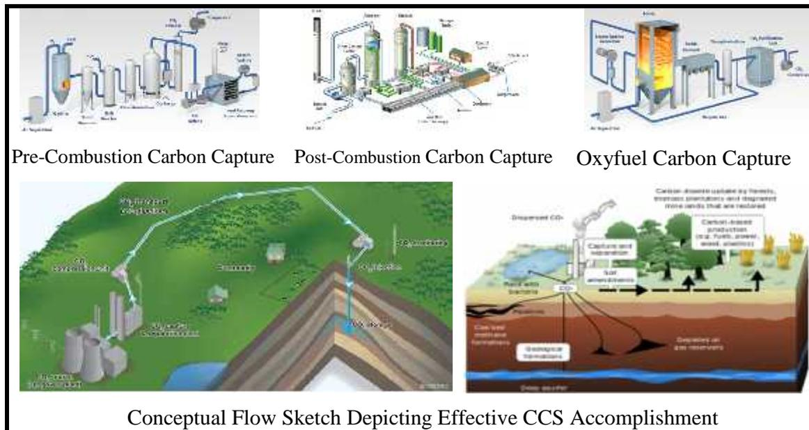
Fig.1 Schematic Drawing of the Carbon Capture and Primary Methods/Processes on CCS
