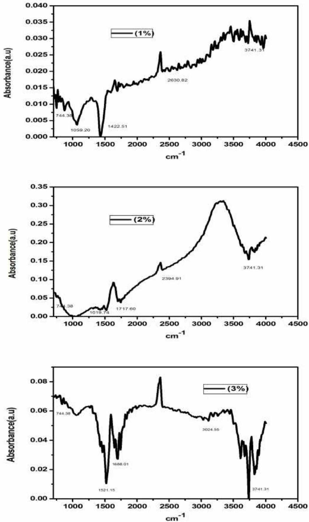
Figure-7 FTIR spectra of Al doped CuO thin film deposited at various weight percentages
