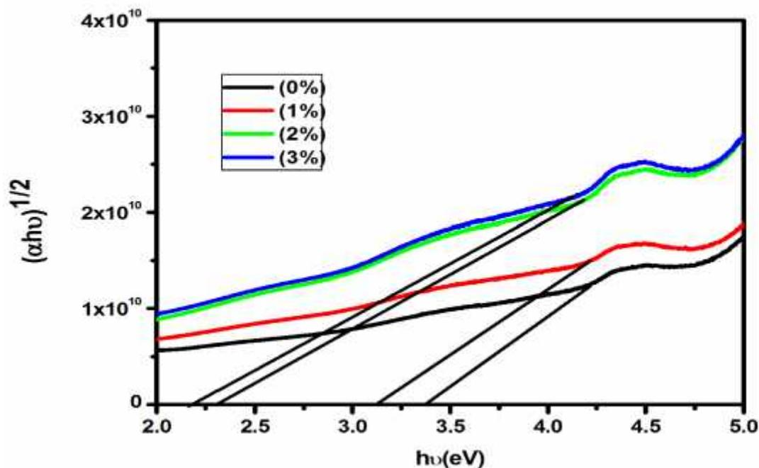
**Figure-5** Optical energy band gap of CuO and Al doped CuO thin film deposited at various weight percentages
