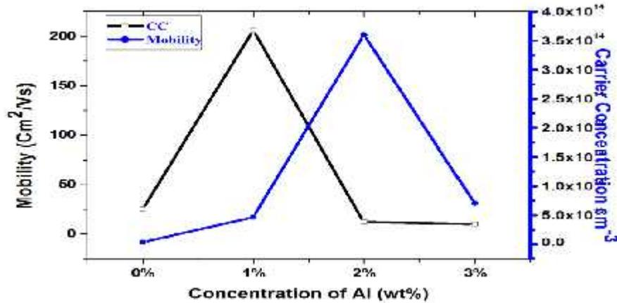
**Figure-8** Mobility and carrier concentration of CuO and Al doped CuO thin films deposited at various weight percentages
