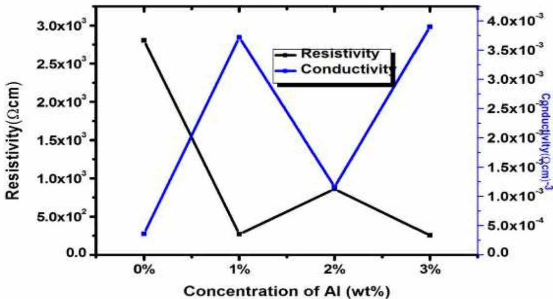
**Figure-9** Resistivity and conductivity of CuO and Al doped CuO thin films deposited at various weight percentages
