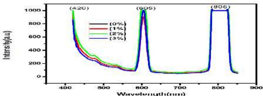
**Figure-6** The PL-spectra of as-deposited Al: CuO on glass substrate at various percentages
