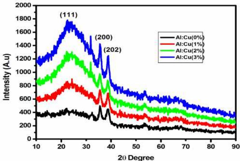
**Figure-1** X-ray diffraction patterns of Al doped CuO thin film deposited at various weight percentages
