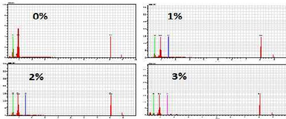
**Figure-3** EDAX spectra of CuO: Al thin films 0%, 1%, 2%, 3% at 400°C
