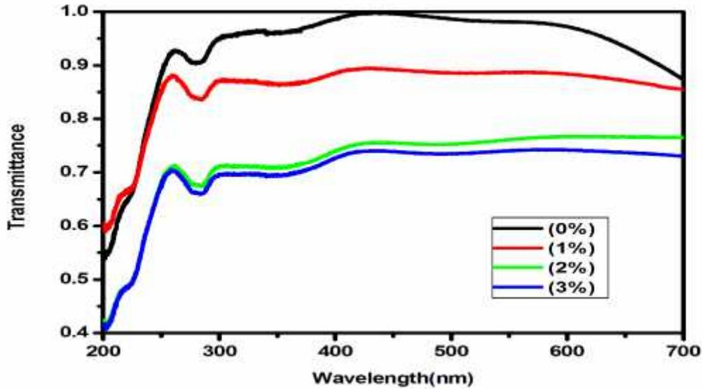
**Figure-4** Transmission spectra of CuO and Al doped CuO thin films deposited at various weight percentages
