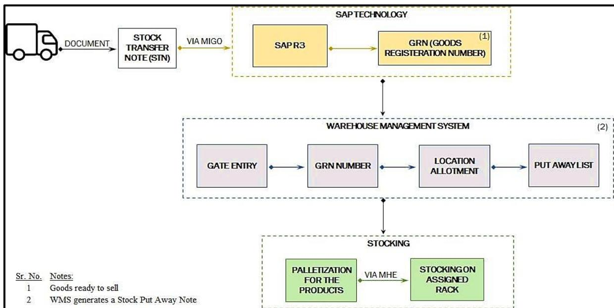
**Figure [3] Inbound Process at Warehouse**
