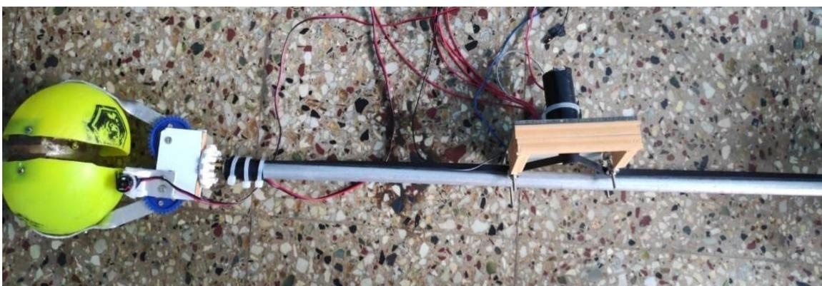
**Figure 5: Robotic arm with gripper**
